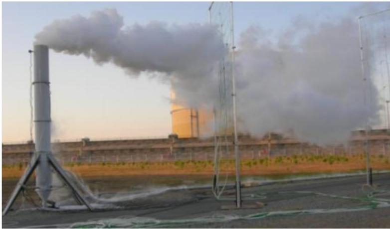
Above - Experimental rig for LNG vapor release (18" vertical plume shown), Ref [1].
